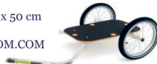
The Y-frame from Carry Freedom is strong as an ox and the best all-around trailer we tested. The Y-frame has an open bed and the trailer is made from a strong aluminum frame covered by a plywood board. It will support about 90kg although this amount is probably not entirely legal. The Y-frame is a bit smaller than the Burley Flatbed but that makes it easier to tow and more stable when weighed down.
